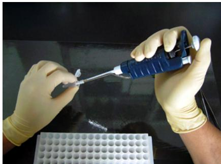
To make **Test Solution**, add **PPV Detection Solution**, **Fluorescent Detection Solution**, and **Enzyme Solution** to a sterilized microtube (0.5 ml or 1.5 ml). Mix the reagents by tapping or vibrating 3 times for approximately 1 second on a vortex mixer, and spin down the tube. It places on ice. Refer also to the following table.
