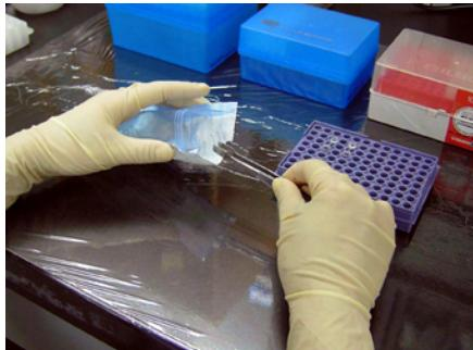
Pick a tube out with clean tweezers, etc. from a bag. Divide 25 µl of **Test Solution** into each **Test Tube**.
