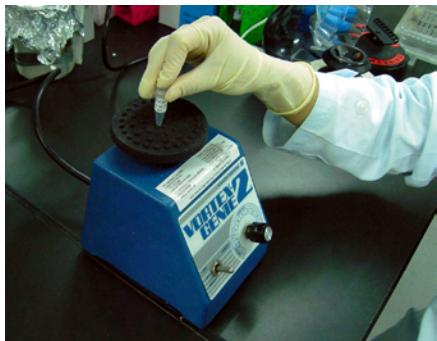
Gently tap the tubes several times (This operation is called tapping.), or vibrate the tubes 3 times for approximately 1 second on a vortex mixer. After the mixture becomes homogenous, centrifuge the tubes to collect the solution at the bottom of the tubes (This operation is called spin down.).
