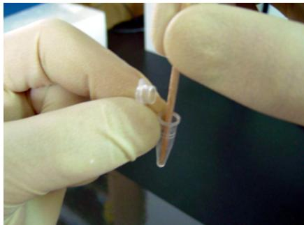
The toothpick which you pricked the leaf, is dipped into **Test Solution**. After all samples are added, 1  $\mu$ l of **PPV Positive Control** will be added to **Test Tube** of **Positive Control Solution**. To prepare **Negative Control Solution**, add sterilized distilled water or nothing instead of sample. Then 20  $\mu$ l of **Mineral Oil** is added to all **Test Tube**.
